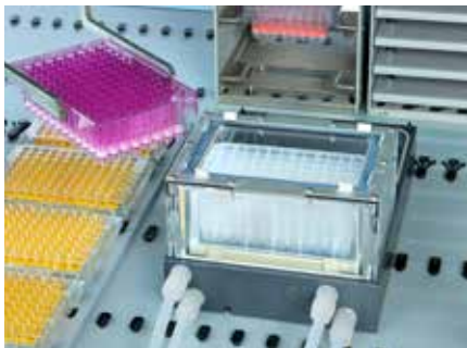
The RoMa moving a new SPE plate to the Te-VacS for subsequent vacuum separation.
