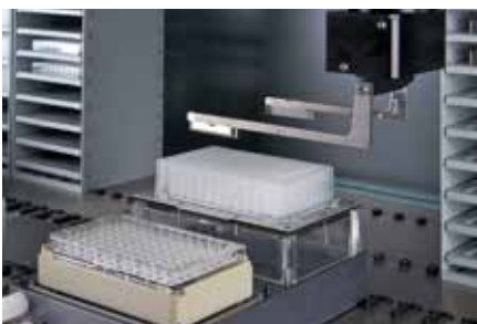
The robotic manipulator arm assembling a Te-VacS™ for a fully automated vacuum solid-phase extraction operation.
