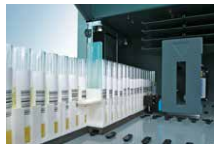
The PosID™ allows barcode identification of tubes or plates.
