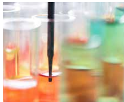
Versatile liquid level detection in individual labware with disposable tips.
