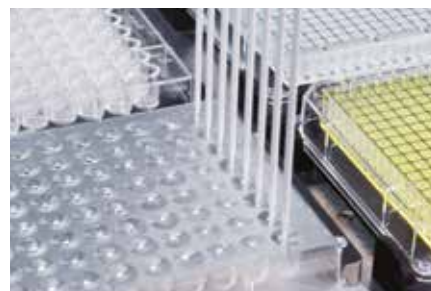
Reliable septa piercing with fixed steel tips enabling long walk away times.
