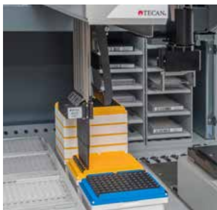
Nested 350 \mu l disposable tips maximize your worktable capacity.
