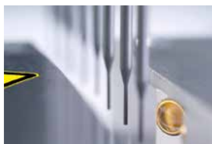
The laser positioning system evaluating tips in-process.
