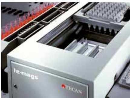
Te-MagS to performs magnetic bead separation.
